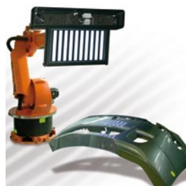
Systems based on the deflectometry principle for the inspection of shiny surfaces Page 12-13
