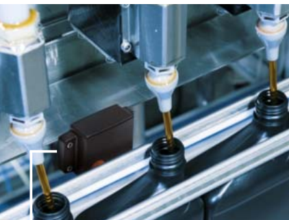
Up to 20 cm: (Ultra) low range antenna for the selective detection of individual products in the close range.
