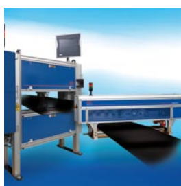
Profilometer for innerliner thickness measurement Page 6-7
