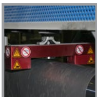
TIP 8301.EO Laser thru-beam / eddy current
