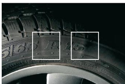
Bulge and dent on a tire surface
