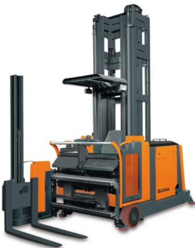
Draw-wire displacement sensors measure the lifting height on fork-lift trucks. You can acquire a lifting heights up to 30 m with this compact construction.
