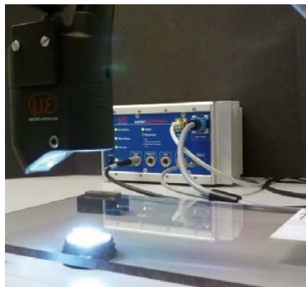
Online measurement of the color gradient of PET and PVC foils/paper.
