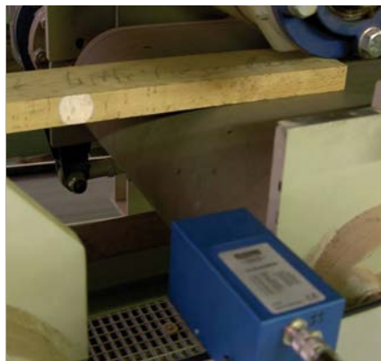
Due to a high rotational speed the wood turns dark. Due to color recognition early in the process, this effect can be compensated for.
