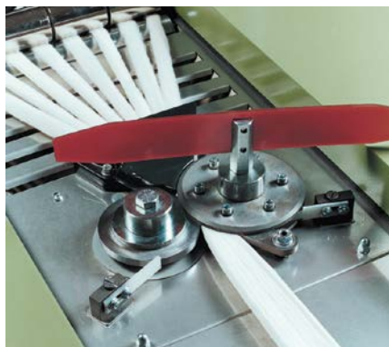
Application in textile machines mainSENSOR measures the rotational speed via small magnets on a wheel
