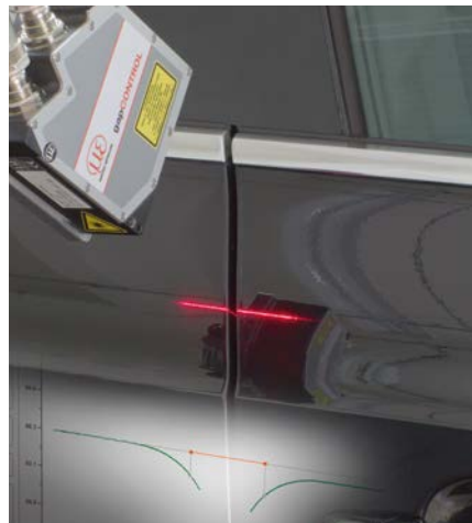
Measuring gaps / flushness for vehicle body parts
